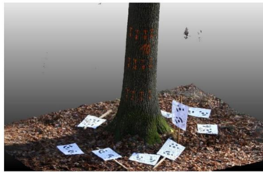
Figure 4. Scaling and orientation process using the coding markers.
