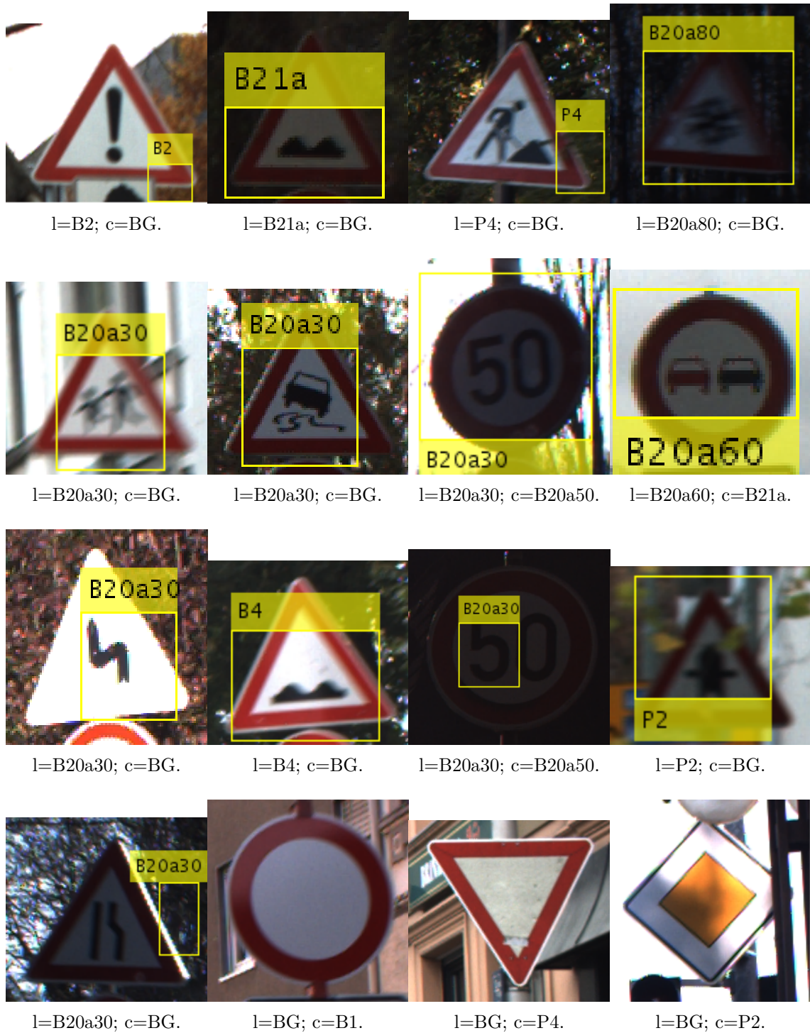
Fig. 3.2: Incorrectly recognized signs; l – label given by detector, c – class of the sign, BG – background
