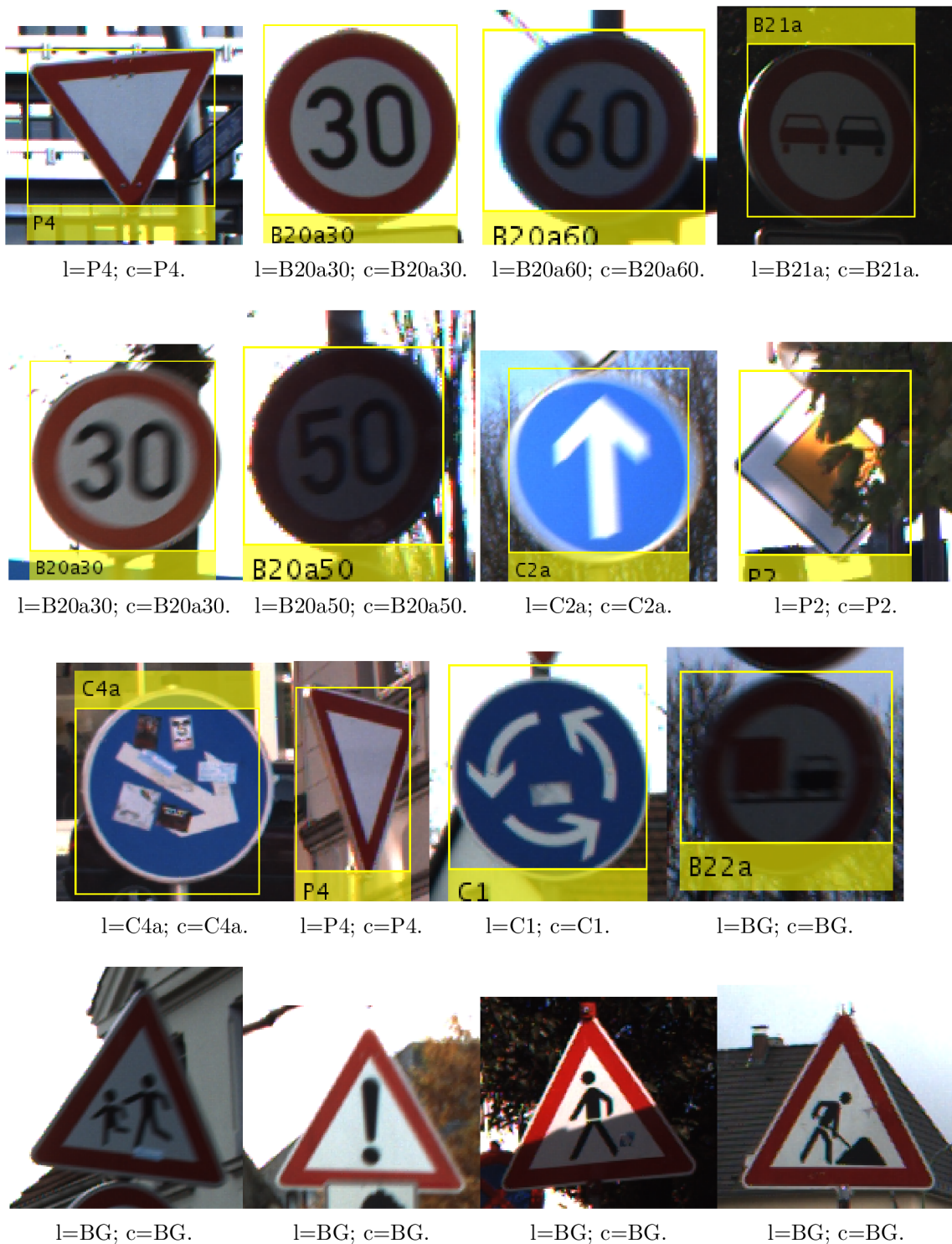
Fig. 3.1: Correctly recognized signs; l – label given by detector, c – class of the sign, BG – background
