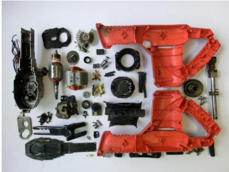
Fig. 6-2 Photography of decomposed Reciprocating Saw (RS1).
