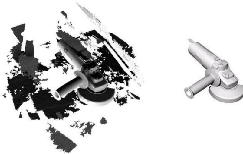
Fig. 5-2 Rhinoceros 7, imported STL Angle Grinder – narex EBU 13; (left) imported model; (right) cleared model.
