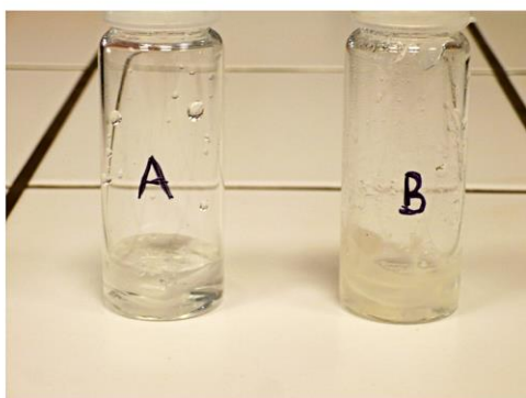
Figure 34. Time dependence of pH of aqueous media during the biodegradation of PLA and PLA-g-IAH at 37\pm 0.1 °C; [IAH]_0 = 0.5, 1 and 5 wt %, [L101]_0 = 0.1, 0.5 and 1 wt % (a); PLA-g-IAH sample before (A) and after (B) biodegradation test (b). contact angle of neat PLA and PLA-g-IAH (c).
