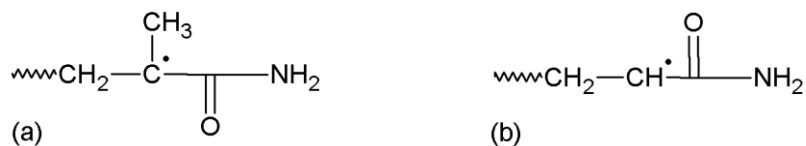
Figure 6. Tertiary (a) and secondary (b) acrylamide radical formed during grafting of cellulose acetate [45].
