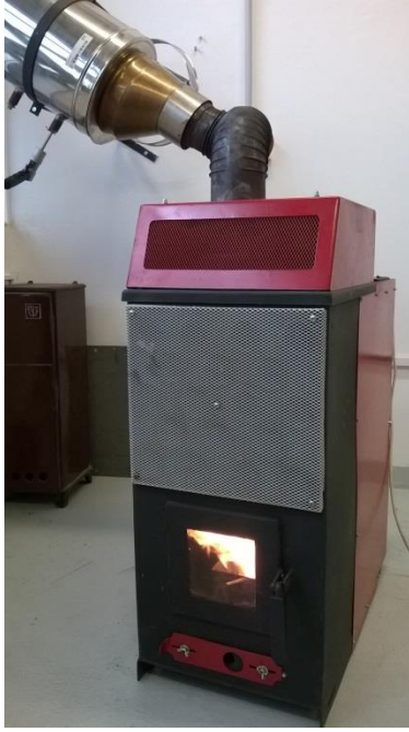
Figure 24. Automatic pellet boiler KNP-18 (Source: Author, 2016).
