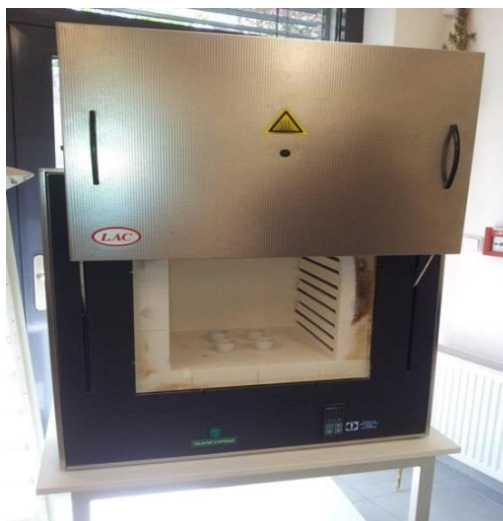
Figure 9. Muffle furnace LAC (Source: Author, 2015).
