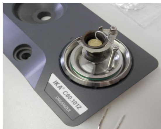
Figure 16. Prepared pellet in oxygen bomb (Source: Author, 2016).
