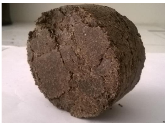
Figure 27. Briquette produced by applying compressive force of 300 kN (Source: Author, 2016).
