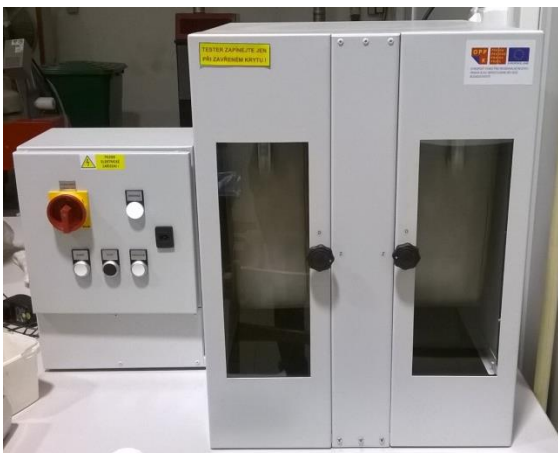
Figure 22. Pellet durability tester for mechanical durability determination (Source: Author, 2016). Figure 23. Pellets in sieve of 3.15 mm (Source: Author, 2016).
