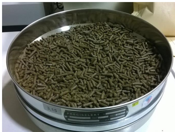
Figure 22. Pellet durability tester for mechanical durability determination (Source: Author, 2016). Figure 23. Pellets in sieve of 3.15 mm (Source: Author, 2016).
