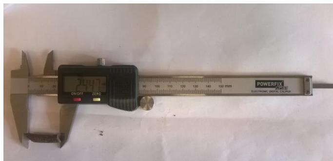
Figure 21. Length determination of pellet by automatic caliper (Source: Author, 2016).
