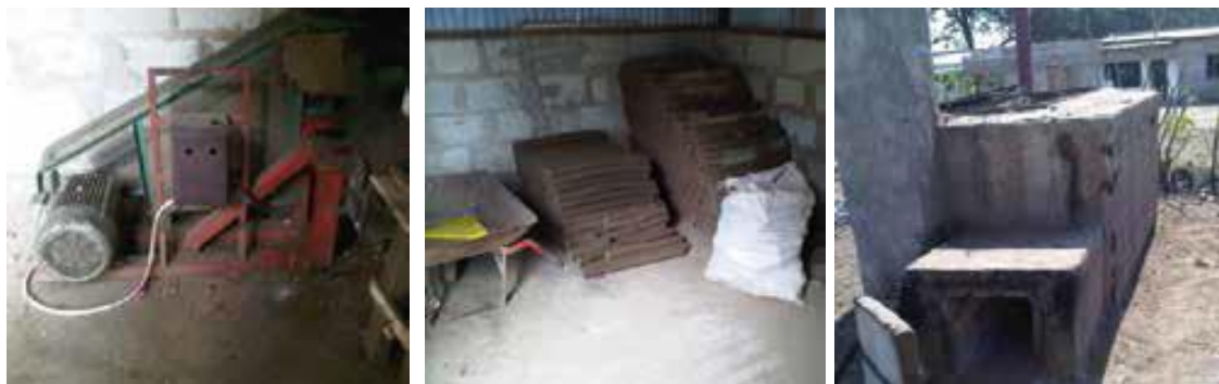
Figure 7. Production of charcoal briquettes in Tanzania: Briquetting machine, Jatropha seed cakes briquettes and Charcoal kiln (Source: Raghavan, 2013).
