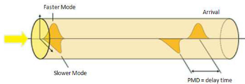
Figure 13: Pulse broadening through polarization mode dispersion
