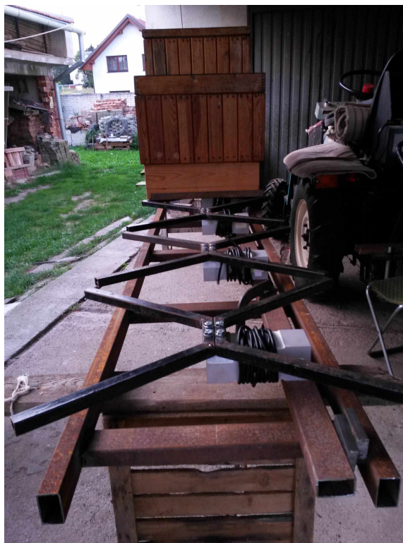
Figure 5.2: Metal platform for eight beehives with Zemic L6G load cells.
