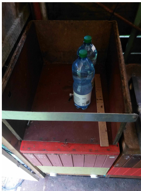
Figure 5.3: Scales for calibration with bottled water.
