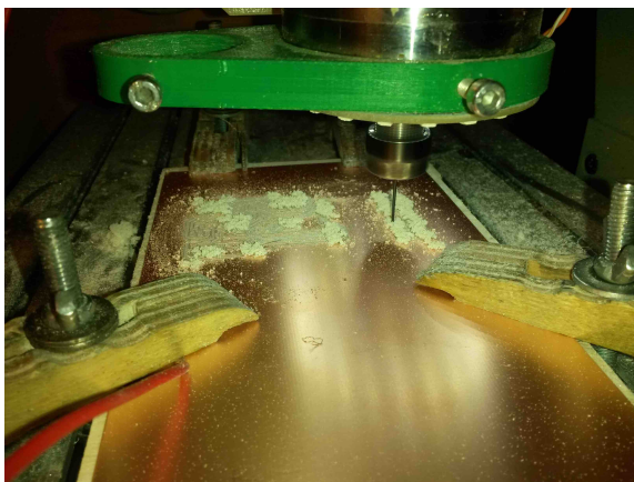
Figure 3.5: Drilling holes of prototype bus-unit board with 1mm drill on a CNC machine.
