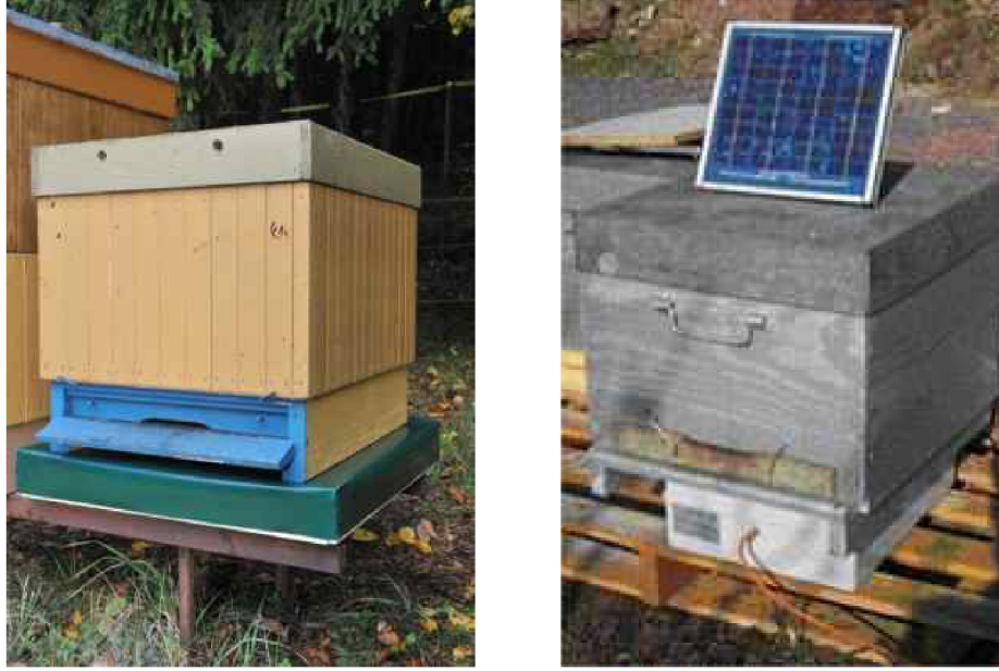
Figure 2.3: Left: Beehive placed on a weighting system of company ALYA s.r.o. [2]. Beehive placed on a weighting system Beewise [5]. (right)
