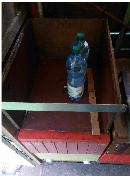
Figure 5.3: Scales for calibration with bottled water.
