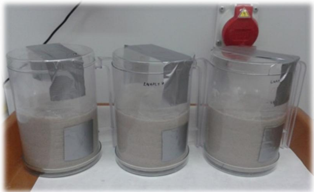
Figure 22 – Packed silica sand columns for experiment
