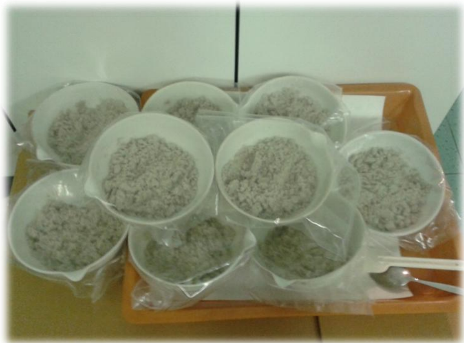
Figure 35 - Homogenization of silica sand and water/LNAPL for sand columns
