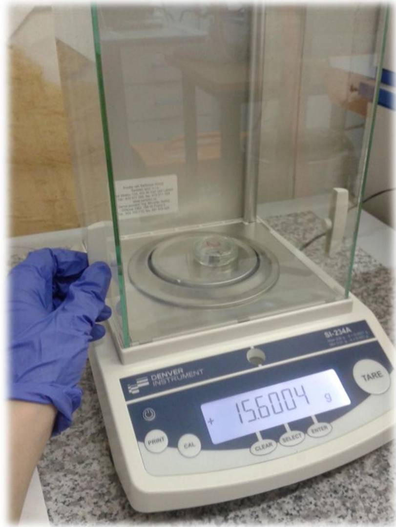
Figure 39 - Taking weight of activated carbon pellets after drying
