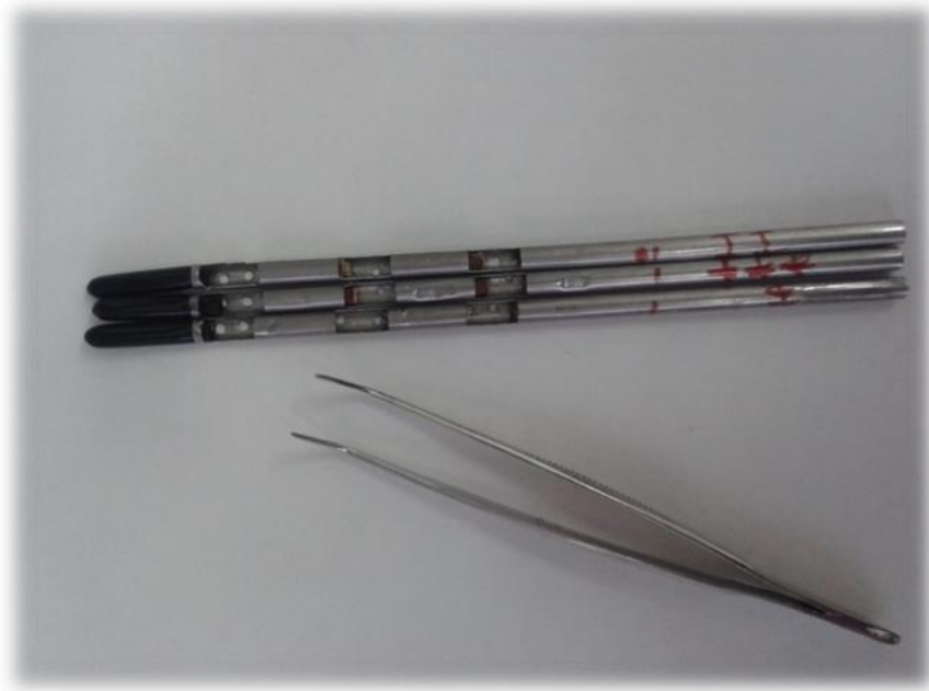
Figure 23 – Stainless steel tubes ready for inserting of activated carbon
