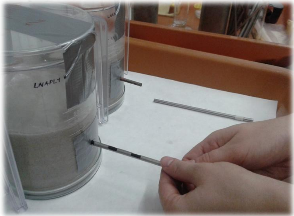
Figure 37 - Inserting stainless steel tube with activated carbon pellets into the silica sand column
