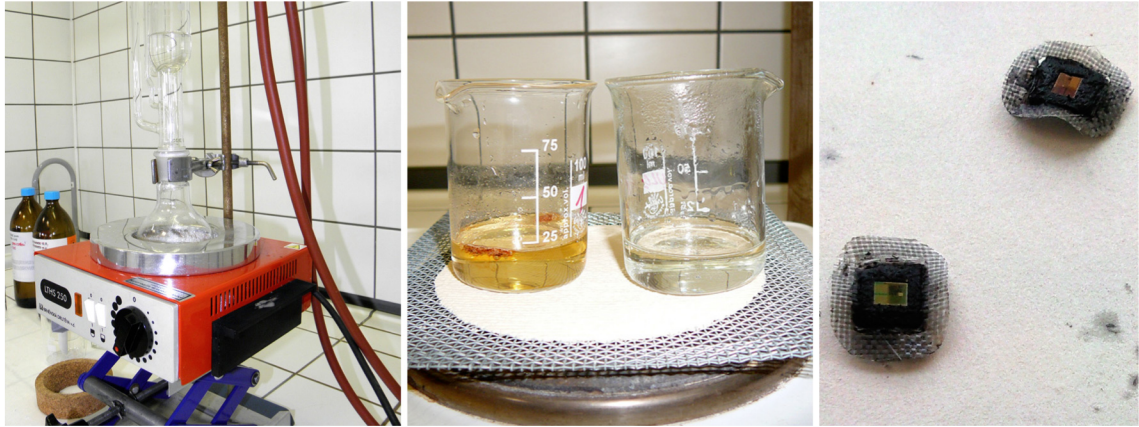
Figure 3.1: Left: Boiling nest with acetone bath. Middle: Two beakers with acids with the decapsulation process is progress in the left one. Right: The result of the decapsulation process—bare chips on their original pads. (Source: author’s work.)
