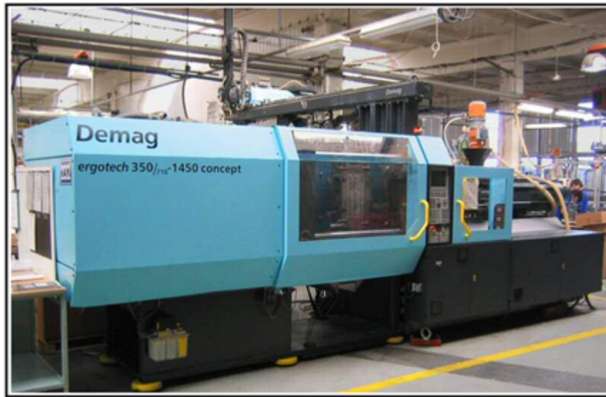
Figure 5-6: An example of a Plastic injection moulding machine. Make: DEMAG, Germany [Source: http://www.plastika.cz/en/photo/002-demag.htm ]
