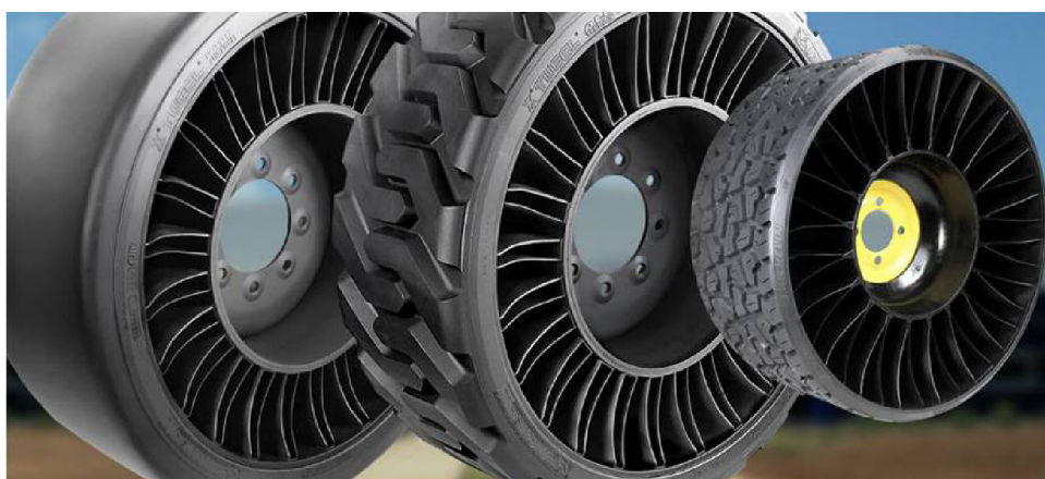
Obrázek 11: Michelin X Tweel. Zleva: SSL All Terrain, SSL Hard Surface, Turf [10]
