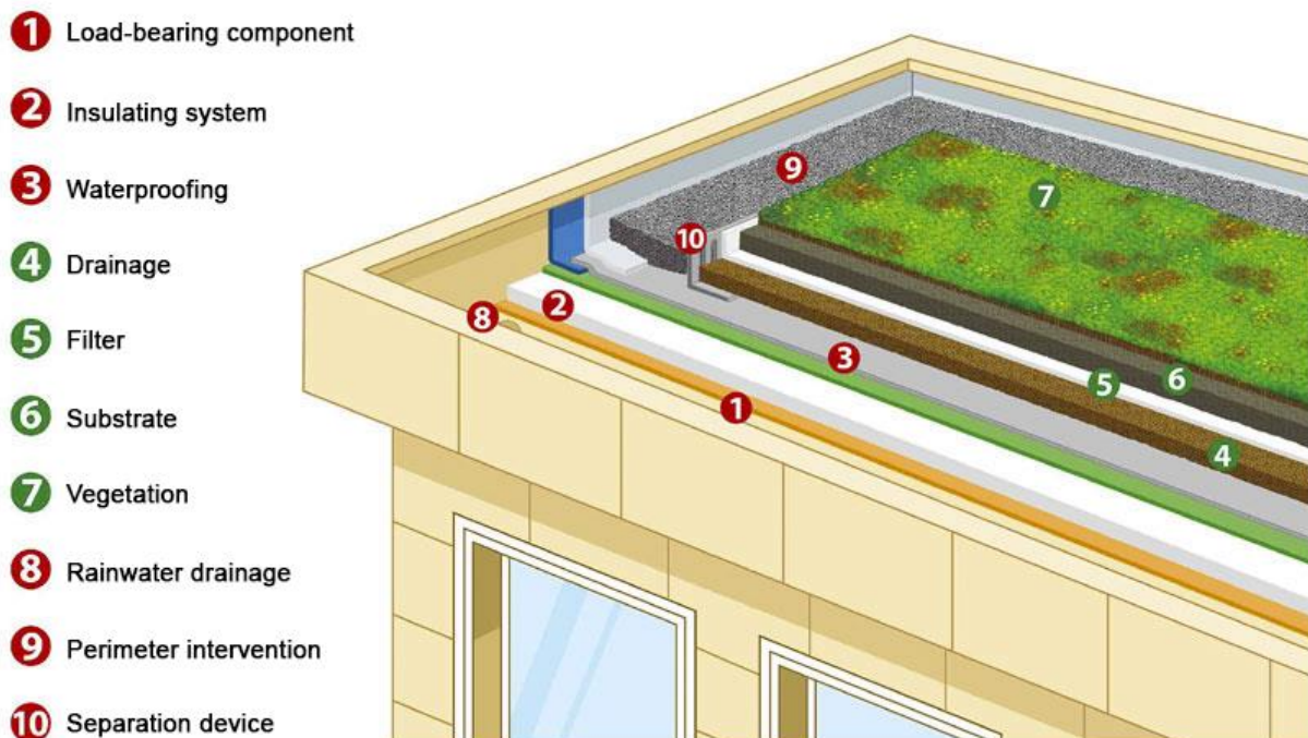
Fig. 12: components of green roof source : https://www.vegetalid.com/solutions/green-roofs/what-is-an-extensive-green-roof/concepts.html
