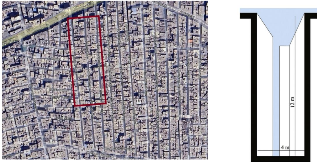
Fig.22 Imbaba – Aspect ratio (H/W=3) building height 12 m street width 4m Source: Google earth
