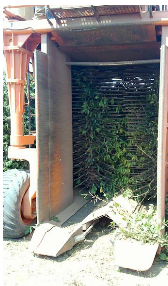
Figure 6 - Tractor with rotating brushes
