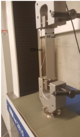
Figure 4.11. The setup of the tensile test
