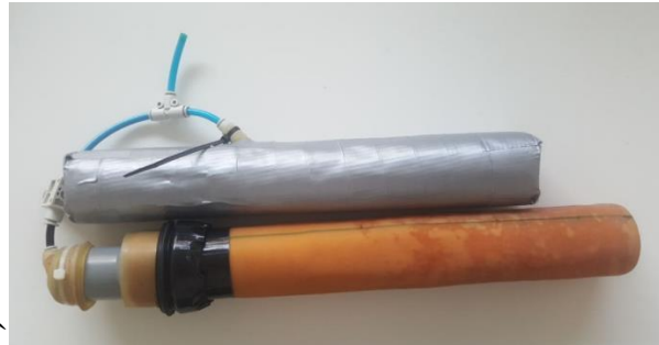
Figure 3.28. The additional latex tube connected to PSE
