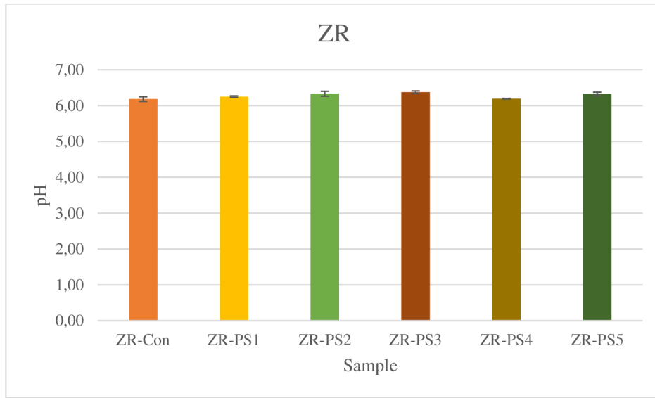
Figure 50 pH measured in water leachates in Zn-rich soil.
