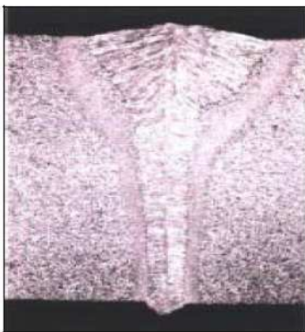
Obr. 21 Svar laser hybridem tloušťka 15 mm [5]
