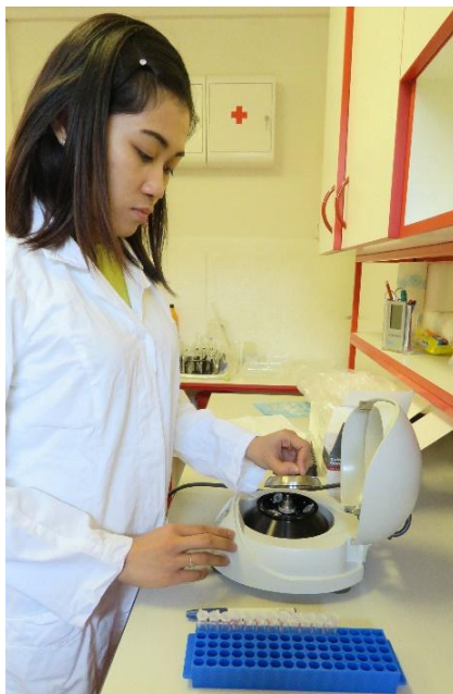
Figure A3.2 Centrifugation of samples at 12,000 RCF for 2 minutes (Photo: Author).
