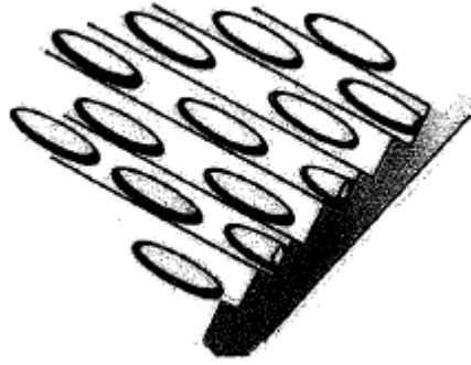
Figure 3: Molecules of LC filling grooves in alignment layer [1].
