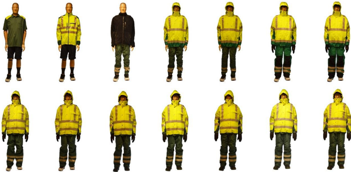
Figure 4: 14 clothing ensembles from Taiga AB (Sweden) with basic thermal insulation from 0.5 to 3.2 clo chosen for the study.
