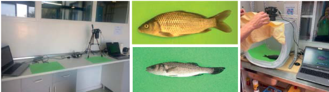
Figure 2. (Left image) seabass data collection design. Digital camera photographing the lateral view of the fish. Image of the seabass (middle, bottom) and carp (middle, top) on the uniform green background. This image was used for automatic fish localization. (Right image) experimental design for carp imaging using a tent with controlled lighting conditions.
