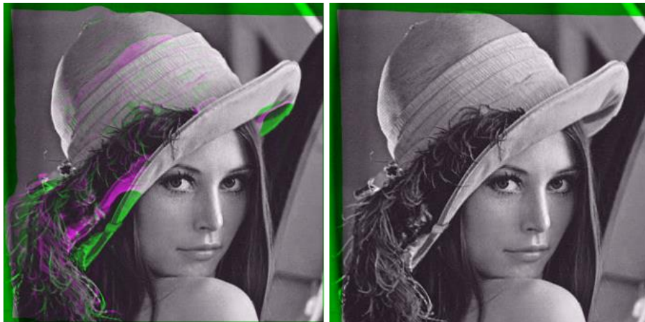
Fig. 7.12 The result of the Demon algorithm. a) 100 iterations, 5 s, quality 0,9559. b) 500 iterations, 27 s, quality 0,9690. See the details in the Tab. 7.2..
