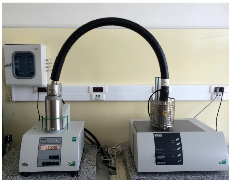
Figure 16 | STA449 C Jupiter-Netzsch connected to QMS 403 Aëolos mass spectrometer (Netzsch).
