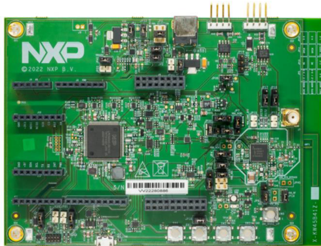
Fig. 1.2 NXP KW45B41Z EVK, taken from [13]
