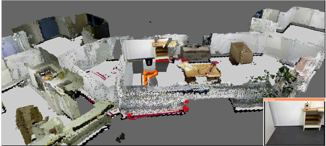
Figure 5.6: Automatically generated and updated 3D model of home-like environment covering an area of 100 \text{ m}^2 .
