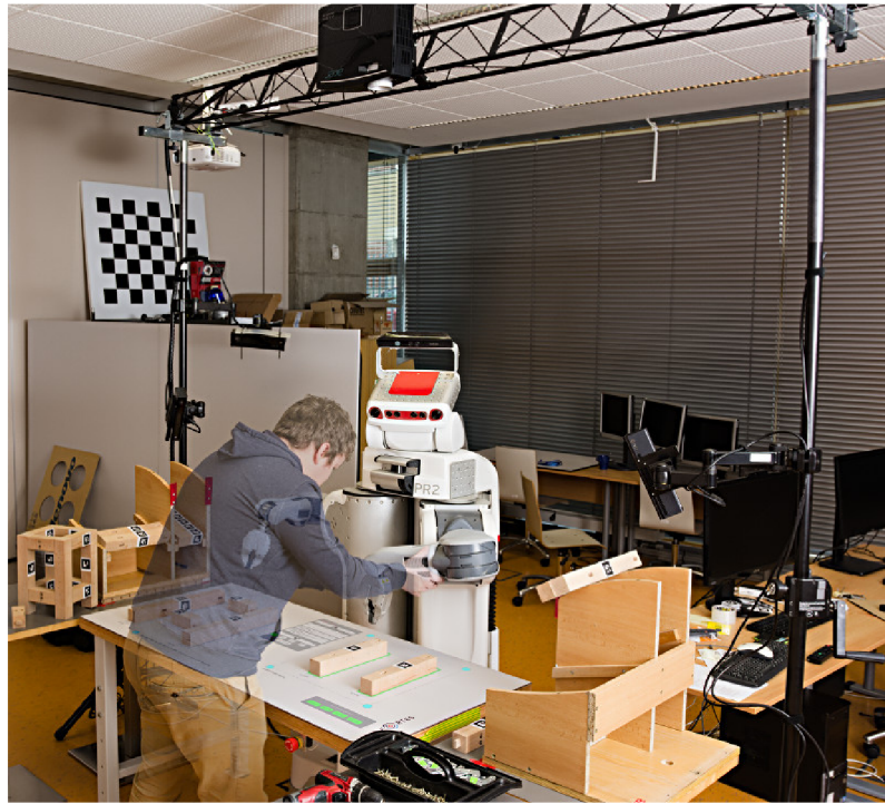
Figure 8.1: Setup of the novel interactive system concept where all the interaction elements (visualization and control) are gathered in a shared workspace (example of setting program parameters using a robotic arm and gestures; image edited).
