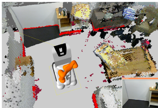
Figure 5.5: The 3D mixed reality environment consisting of a robot model, 2D laser data, a 2D map, a combination of the live RGB-D data in current field of view of the robot (visualized using yellow lines) and the 3D voxel-based map outside it and a video stream.
