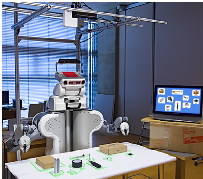
Figure 6.1: Prototype of the human-robot shared-space environment with augmented reality user interface (image edited).
