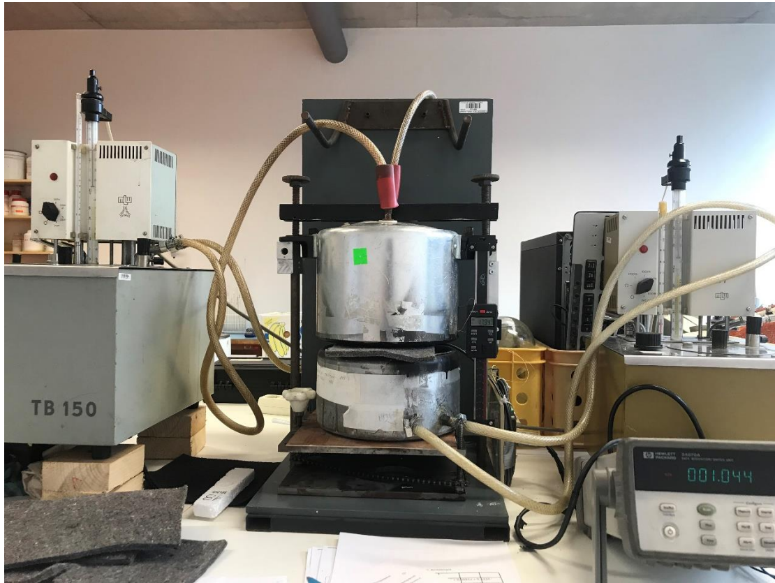
Figure 9: shows the exact experimental setup as described in the figure above and how the sample testing is done to find effective thermal conductivity.
