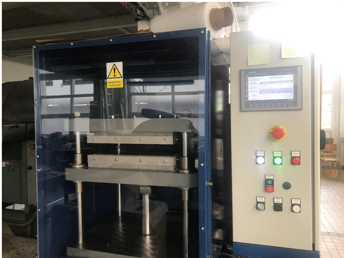
Figure 11: represents the picture of hot pressing machine in our laboratory which is used for the drying of the samples at high temperatures.
