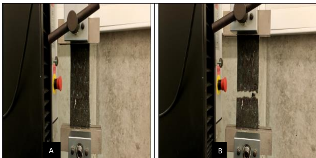
Figure 21: (a) represents the sample in the tensile testing machine before stretching. (b) represents the sample after fully stretched to the maximum point in the tensile testing machine.
