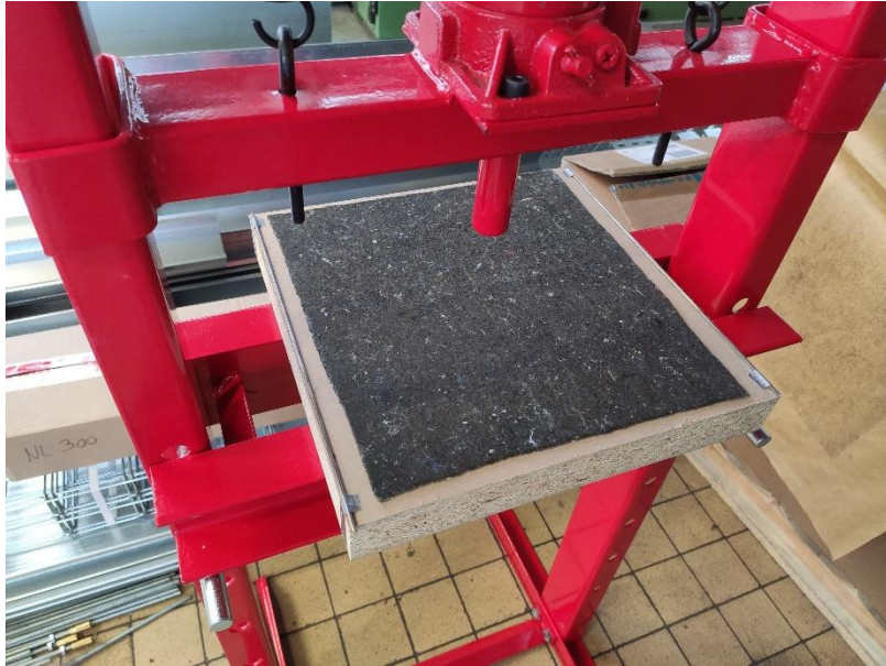
Figure 12: represents the cold pressing machine with the sample on it
