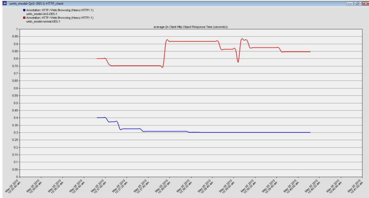
Figure 4-17 Web response time at HTTP_client
