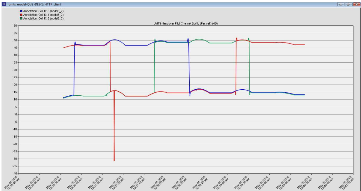
Figure 4-18 Softer handover on mobile client
