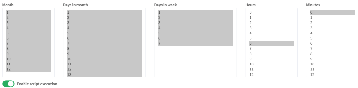
Figure E.1: The CRON settings dashboard showing the CRON job will be executed every day of the month at 6 AM.
