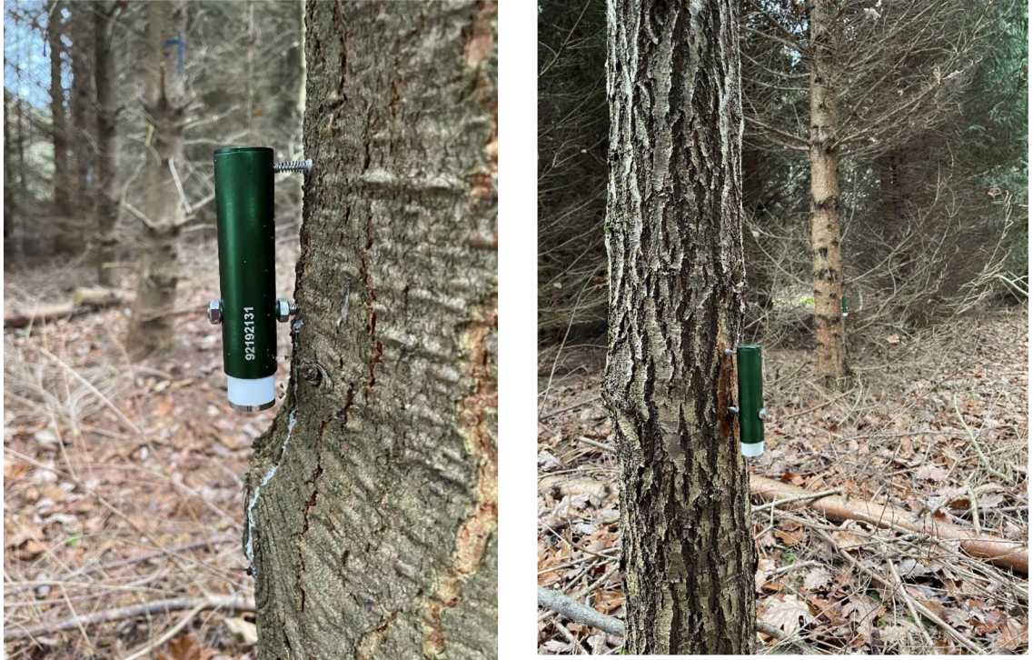
Figure 4. Tomst dendrometers installed in Kaltenborn study site. From: Radim Matula
