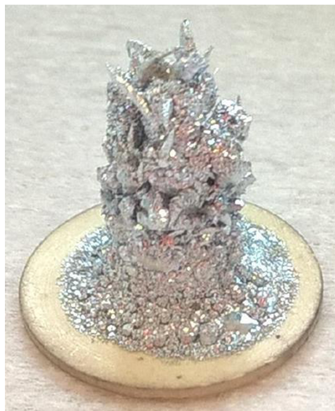
Fig. 68: A lid of the Zn effusion cell blocked with zinc deposits.
