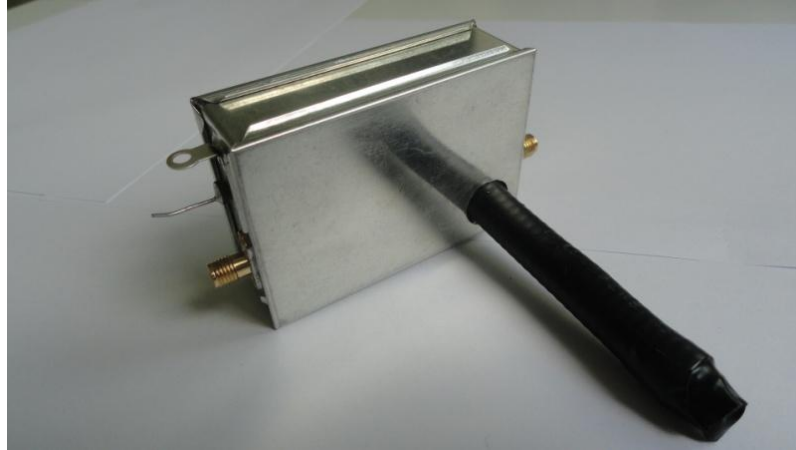
Figure 2.26: Low Noise Amplifier for UHF Band (430-440 MHz).
