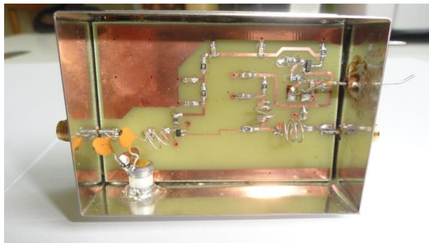
Figure 2.25: Implementation of the LNA with FR-4 substrate.
