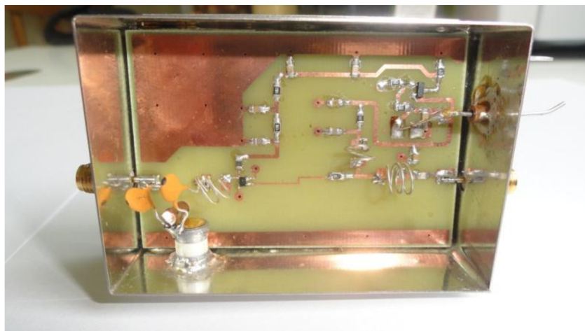
Figure 2.25: Implementation of the LNA with FR-4 substrate.
