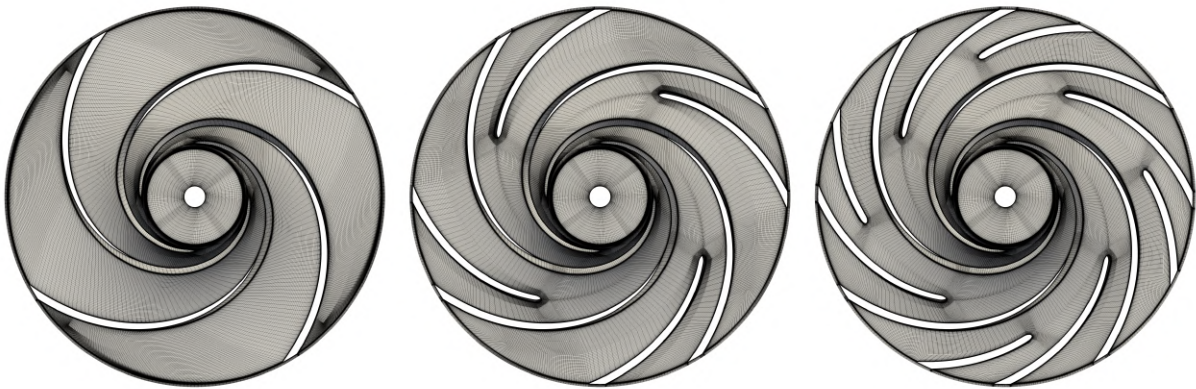
Figure 4.20: View of the impeller grid for Case 0sp, Case 1sp and Case 2sp.
