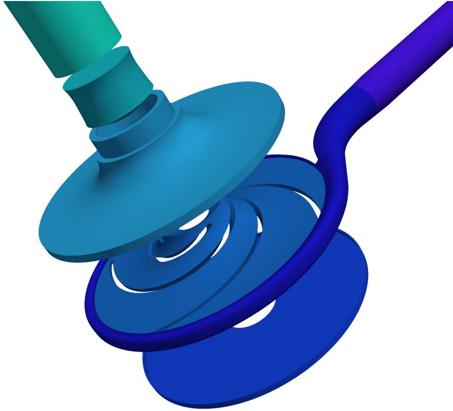
Figure 3.9: Decomposition of the pump into numerical domains.
