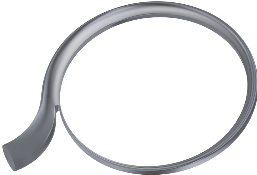
Figure 2.10: Volute at a specific speed n_s = 32 .
