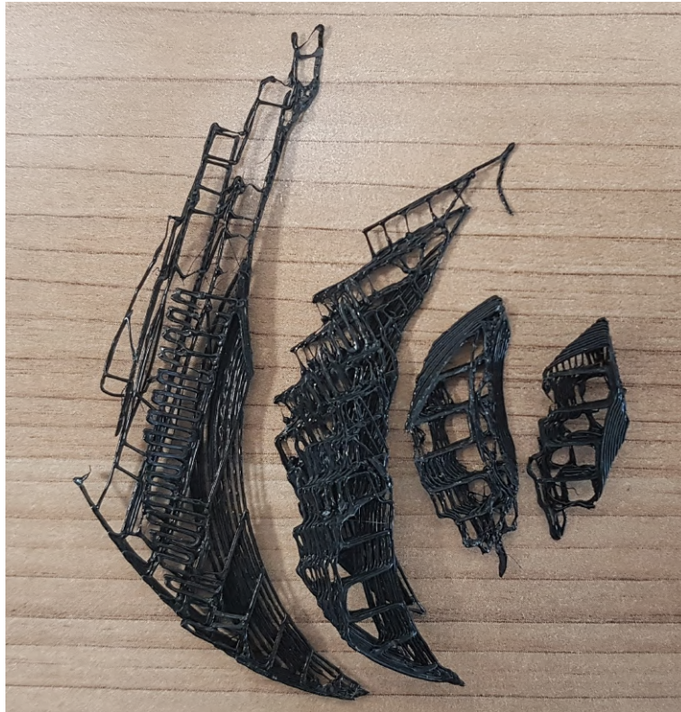
Figure 3.18: Impeller 3D printing supports inside channels due to insufficient time in the solution of sodium hydroxide.
