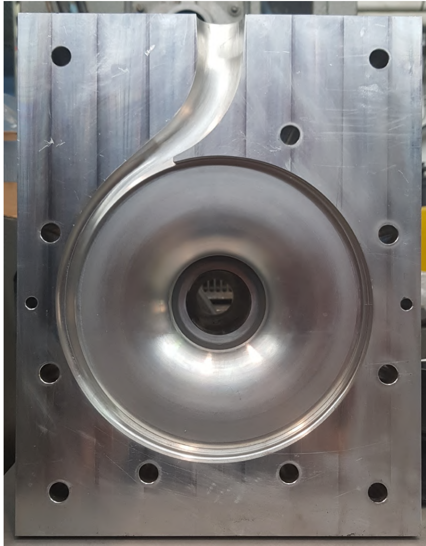
Figure 3.17: Casing (Hub side).
