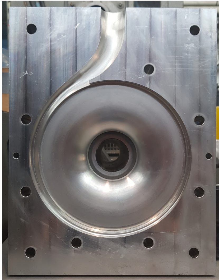
Figure 3.17: Casing (Hub side).
