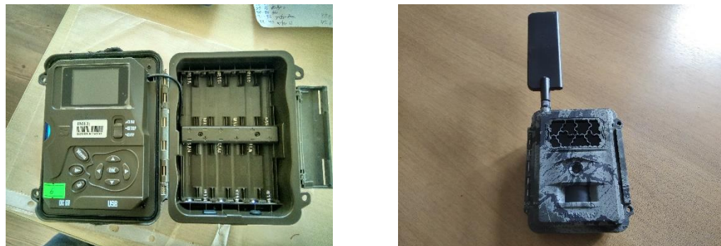
Figure 24. Camera traps for determination and monitoring of forest conditions, pictures taken in Borjomi-Kharagauli National Park, Georgia (2022)
