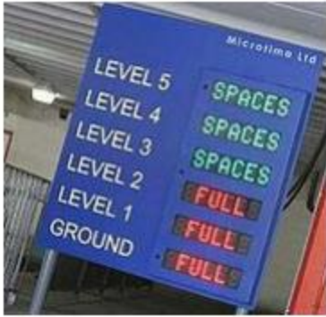
Figure 5: Display Board at Parking Entrance
