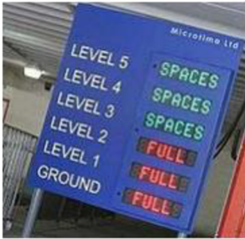
Figure 5: Display Board at Parking Entrance
