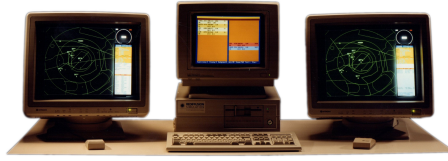
Figure 2.6: Micro Nav's first generation of Air Traffic Control simulator [17].
