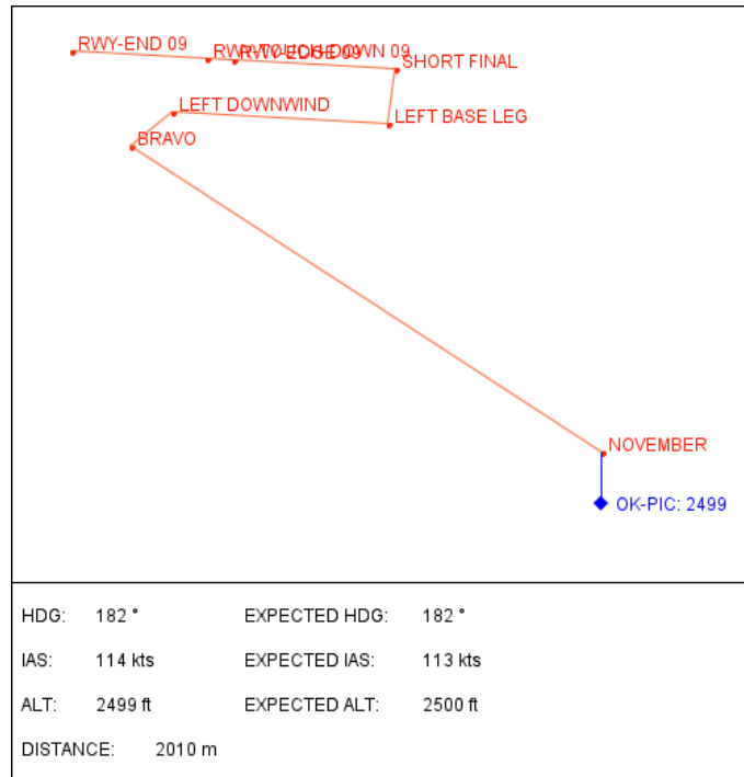
Figure 5.21: Screen for visualization of pilot's tasks and planned trajectory.
