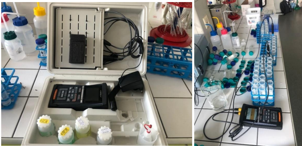
Figure 10 – Multi-parameter device Multi 3620 IDS SET C / Determination of pH and conductivity of water samples.
