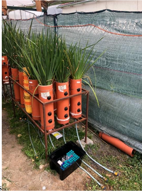
Figure 9 – The sub-surface constructed wetland setup simulation in the Czech University of Life Sciences, Prague
