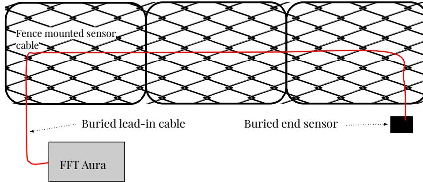
Fig. 6.1: Future Fiber Technology Aura system deployment [30]
