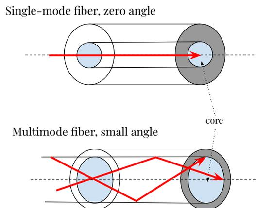
Fig. 2.2: Light propagation in the fiber [2], [9]
