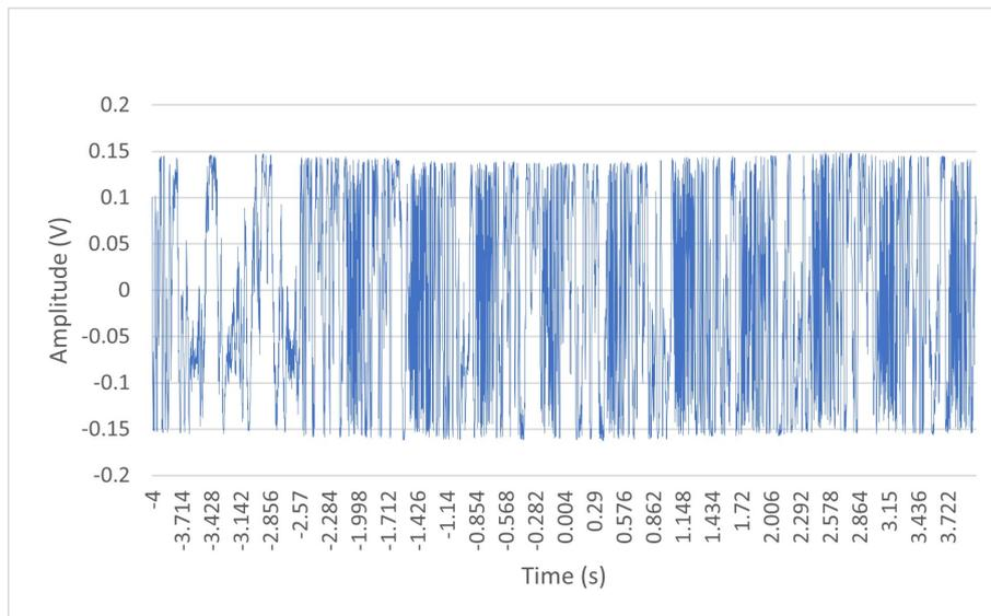
Fig. 7.4: Jumping on the ground where sensing cable is located
