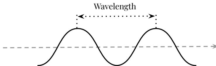
Fig. 1.1: Wavelength shown on sine wave [3]
