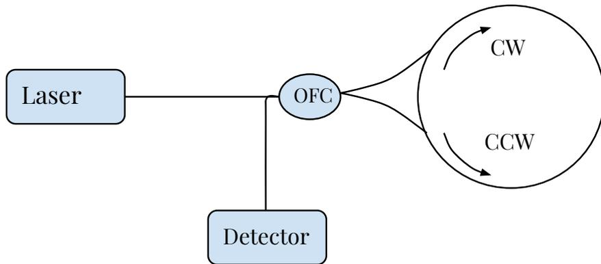
Fig. 5.4: Sagnac Optical Interferometer construction [20]
