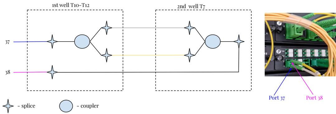
Fig. 7.6: Mach-zender interferometer-based system for the practical section
