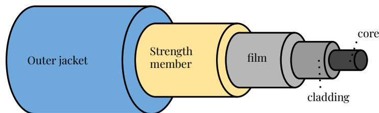
Fig. 3.1: Simple fiber optic cable structure [10]
