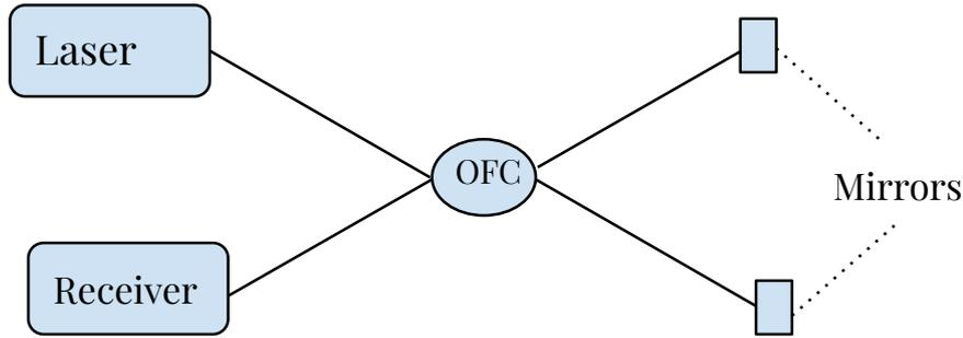
Fig. 5.3: Michelson Optical Interferometer construction [20]
