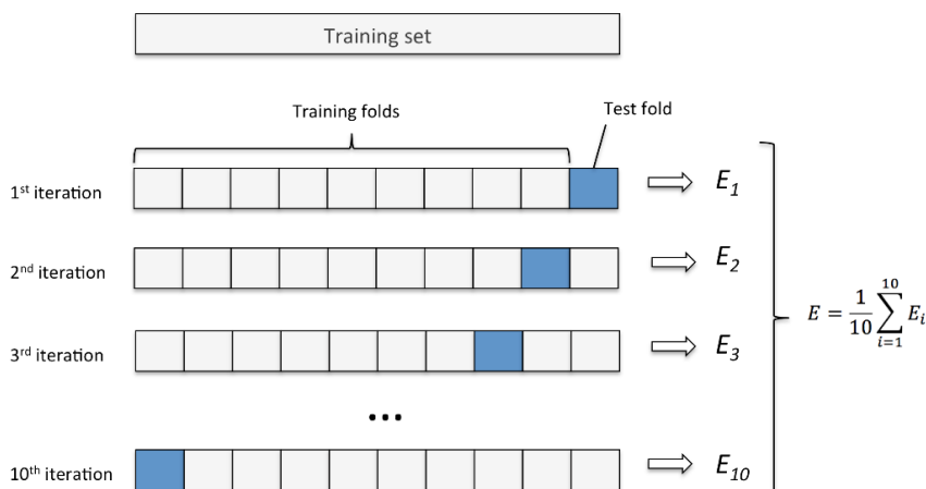
Figure 2.8: k-fold Cross-validation with k = 10 [10].
