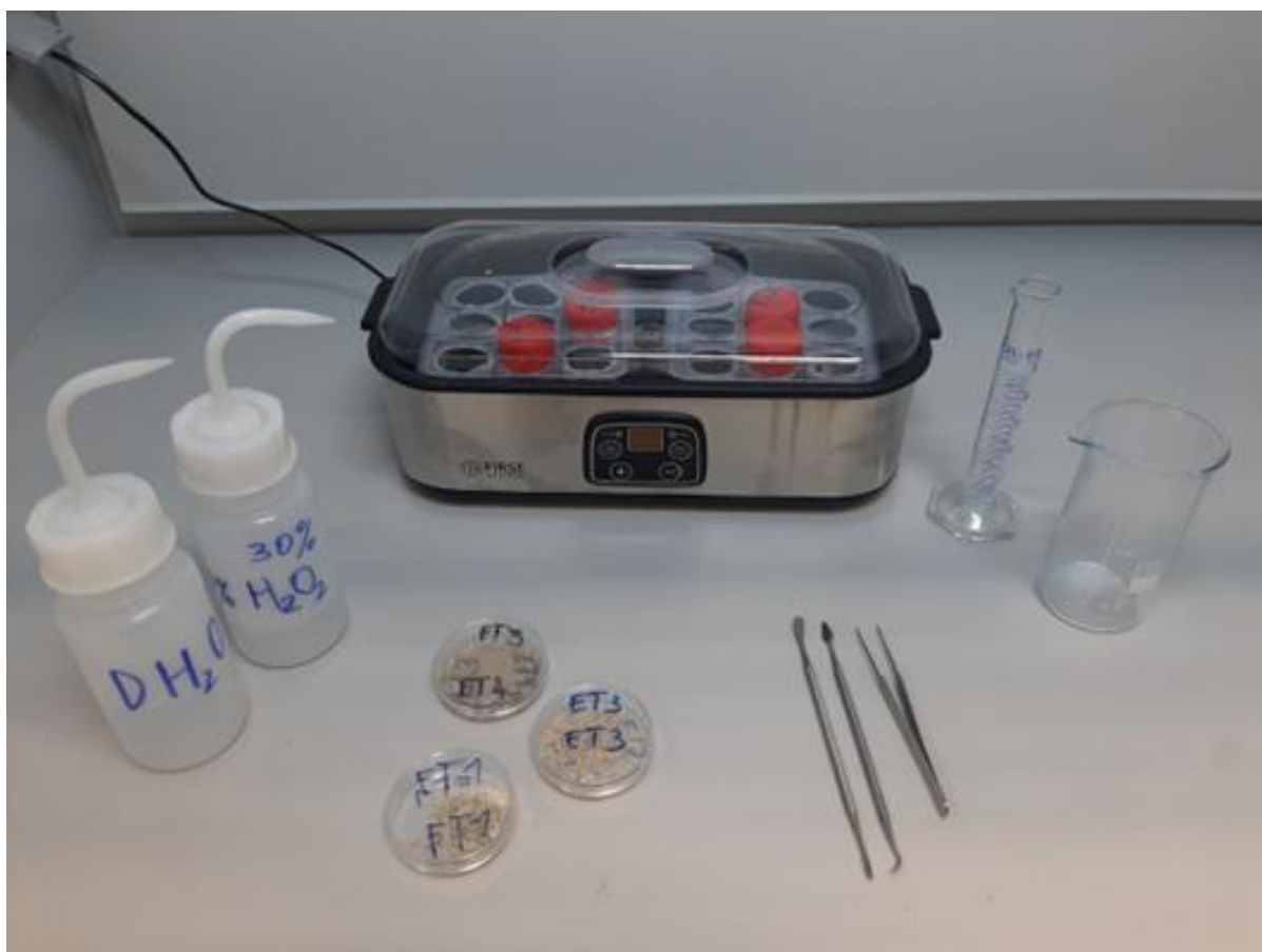
Figure 17: Organic matter dissolution setup
