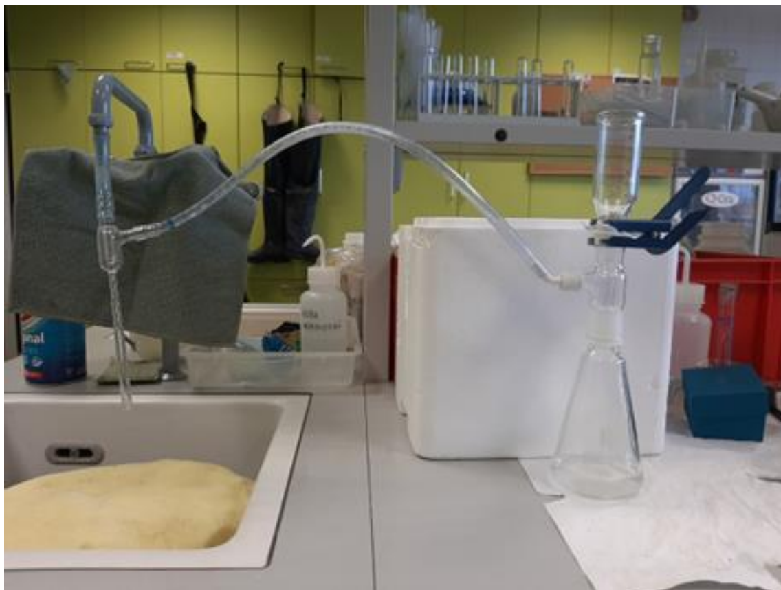
Figure 12: Vacuum Filtration Apparatus with Water Aspirator Attachment at the Hydrobiological laboratory, Czech Republic.
