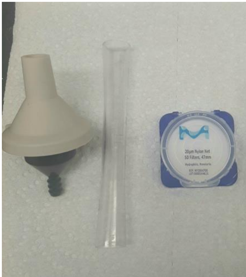
Figure 10: A manual filtration setup used for processing microplastic samples in Guam. The setup includes a mesh filter, a collection container, 20-micron nylon filters, and a tube.
