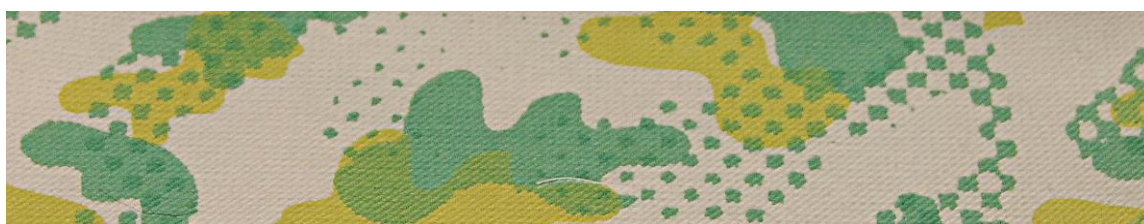
Figure 11 Photochromic pigments ranges 1:4 Y/B and 4:1 Y/B applied on 100% ecru cotton denim textile surface after UV irradiation in presence D65
