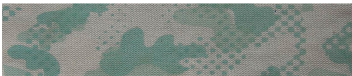
Figure 9 Photochromic pigments ranges 1:4 Y/B and 4:1 Y/B applied on 100% ecru cotton denim textile surface without influence of UV irradiation
