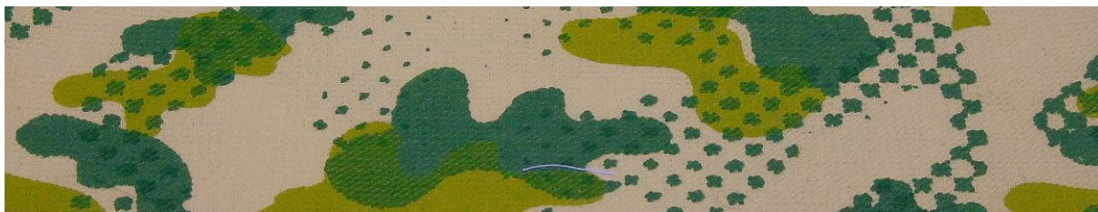
Figure 10 Photochromic pigments ranges 1:4 Y/B and 4:1 Y/B applied on 100% ecru cotton denim textile surface after UV irradiation in dark room
