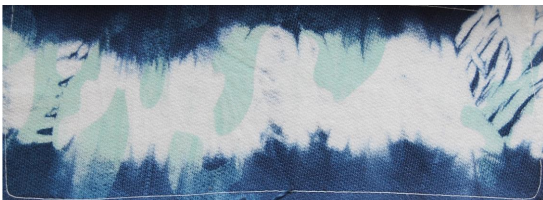
Figure 12 Photochromic pigment range 1:4 Y/B screen printed on 100% cotton knit and then shibori dyed in IBERIA CLASSIC textile dye in navy colour.
