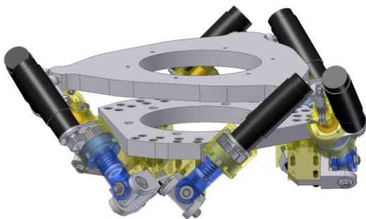
Fig. 5.3 The designed Stewart platform – 3D model (by Houška, P.)
