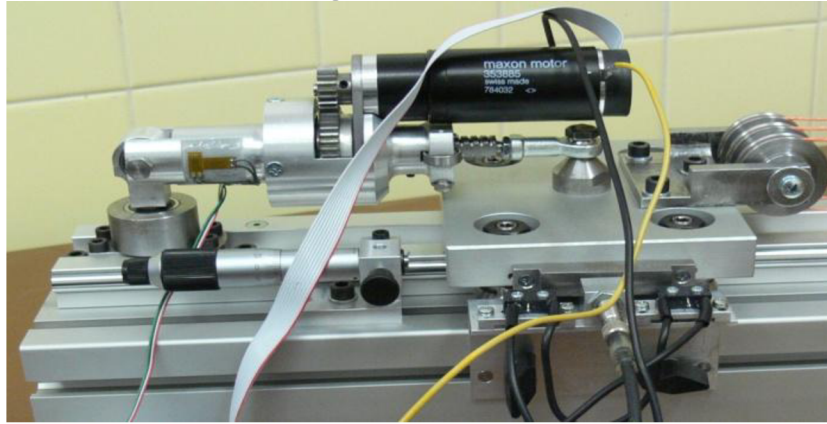
Fig. 10.1 Test jig with the linear actuator
