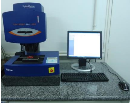
Obr. 9: 3D profilometr Talysurf CLI 1000
