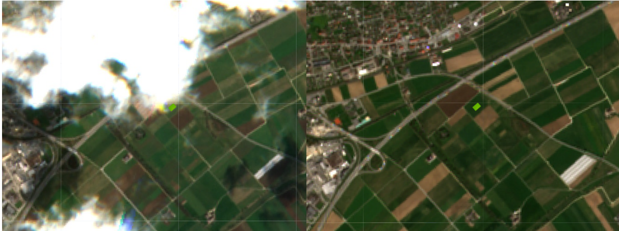
Figure 5.3: Cloud masking application on an image from 14th April 2022. Left side - image before cloud masking was applied, right side - image after cloud masking was applied. The Oensingen study site is depicted in green color.
