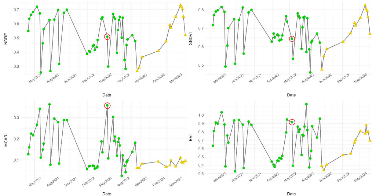
Figure 6.4: First row left to right: time-series plot of NDRE, GNDVI. Second row left to right: time-series plot of MCARI, EVI. The values from 14th May 2022 are circled. While there is a decrease in NDRE and GNDVI due to the rain, MCARI and EVI are not affected.
